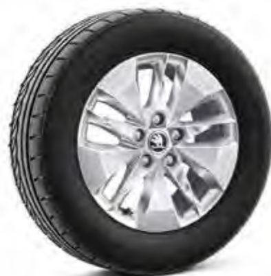
Kola z lehké slitiny TWISTER Aero, 16" (disk: 7J × 16" ET46, pneu: 205/60 R16)
