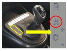
For AMT (Automated Manual Transmission) vehicles, move the shift lever to the N position.
